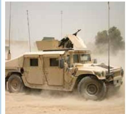
NP Aerospace has developed and manufactured armour solutions which are typically more than 40% lighter than an equivalent performance armoured steel solution by integrating high-technology ceramic and composite materials.
