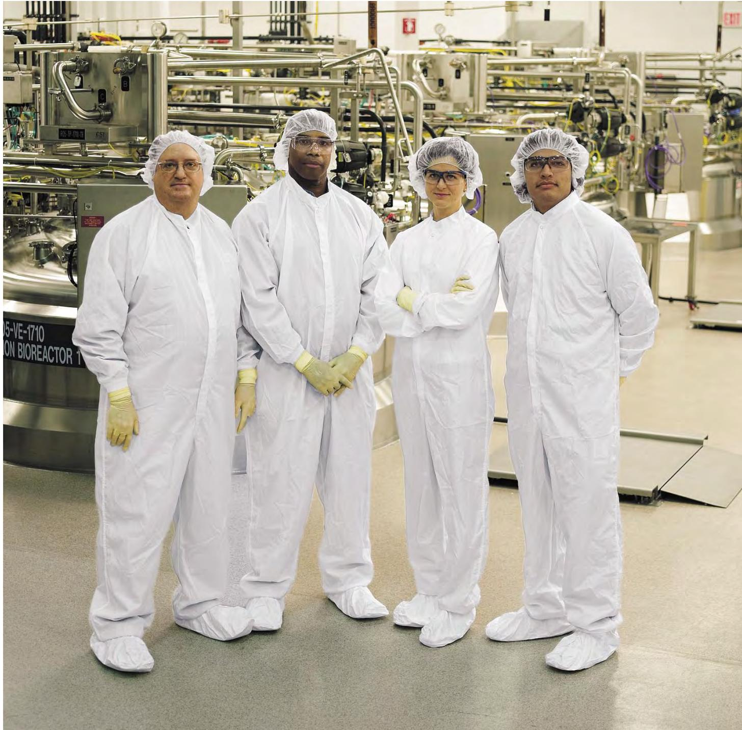
**Amgen Rhode Island manufacturing staff members stand in front of 20,000-liter cell culture bioreactors at the company's new plant in West Greenwich, Rhode Island. The bioreactors, used to manufacture Enbrel® (etanercept), are among the largest in the world.**
