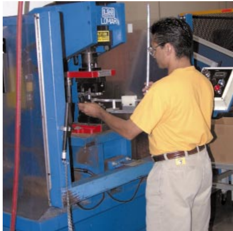
Jerry Perez operates equipment used to crimp a hose to the end of a tube – a hose assembly product that was new to the Bowling Green hose plant in 1999.
