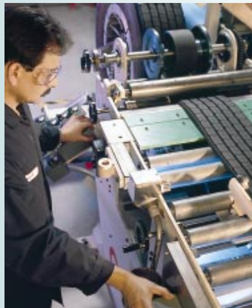
Bruce Alexander, at the Athens technical center, demonstrates Oliver's latest tread builder which applies precise tread rubber and bonding gum in one step to a professionally-prepared and inspected radial truck tire casing.
