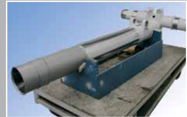
B-777 nose landing gear piston
