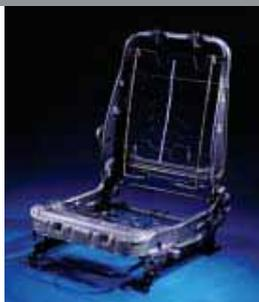
Kobe Steel's high strength steel sheet has enabled car manufacturers to reduce the weight of cars and offer protection to drivers under crash conditions. The Company has commercialized in rapid succession an extensive lineup of high strength steel sheet.
