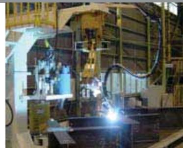
Kobe Steel has developed this innovative proprietary system as a comprehensive welding solution. It features automated welding of joints, a process stage where it has not been possible to use welding robots.
