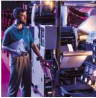
Batavia Plant Manager Jeff McVicker oversees production of a roll of pressure-sensitive labels as it comes off the flexographic press
