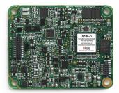
Signal processing apparatus for all Masimo technology platforms
