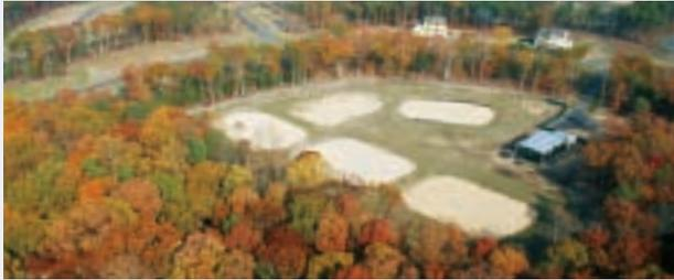
*Wastewater is treated through a membrane bio-reactor process which treats water to a high level effluent quality. Effluent is disposed through rapid infiltration basins, a land based disposal alternative that recharges aquifers and ensures groundwater is a renewable resource for future generations.*
