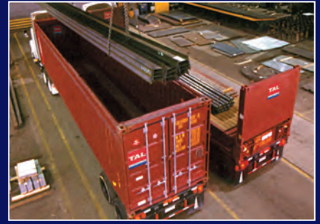
Special Containers – Open-Top Container (left) and – Flat-Rack Container (right)
