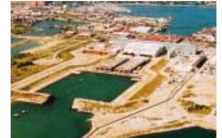
1 The Øresund Tunnel's 20 concrete elements, each weighing 55,000 tonnes and the size of two football pitches, are manufactured in a purpose-built factory
