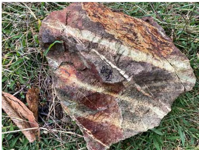
Honeysuckle Prospect: Outcropping altered and veined felsic intrusive rock
