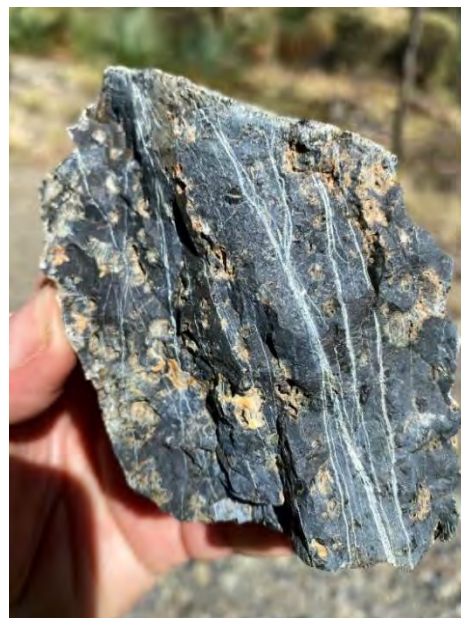
Campbells Prospect: Samples of the chromite mineralised serpentinised ultramafic
