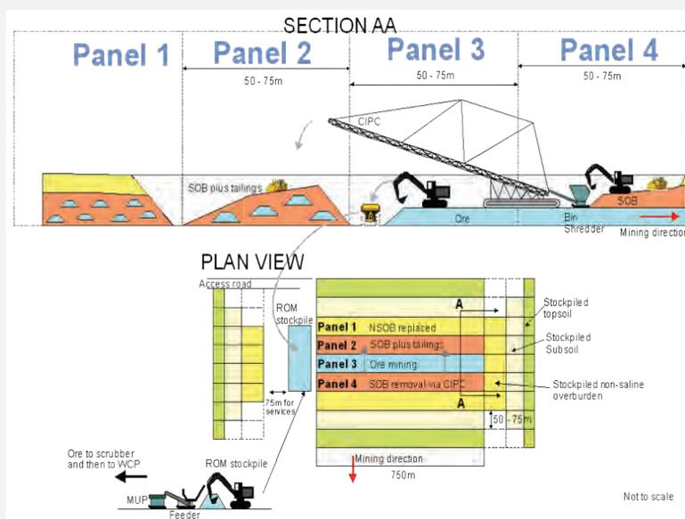
The initial 3 months of operations, overburden will be stockpiled outside the pit. Once the pit is large enough to host the full complement of earth moving equipment, overburden will be direct deposited into the pit void.
