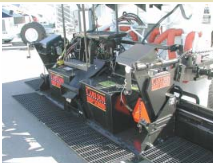
Carlson EZ III™ screed has been updated to a new 34 kW generator for faster heat-up time.
