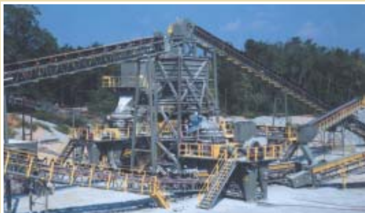
52SBS and 57SBS cone crushers arranged on modular structures to share a common discharge belt.
