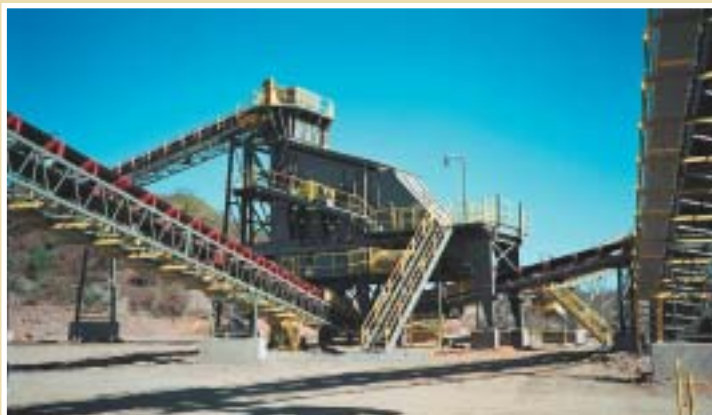
Modular screen tower for a Tel-smith 8' x 20' triple deck screen utilizes roll-away chutes.
