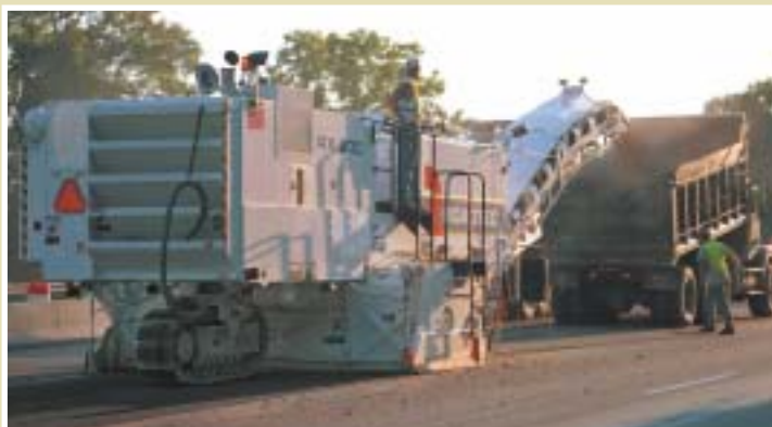
The RX-60 C is a high-horsepower, high-production cold planer that easily converts from half lane to full lane, providing excellent productivity and reliability in either configuration.
