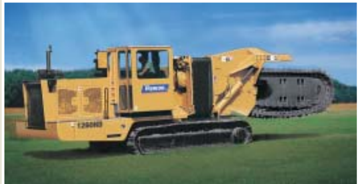
The Trencor 1260 HD trencher can cut trenches up to 12 ft. deep and 42" wide.
