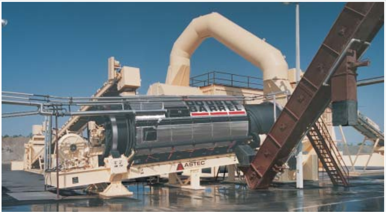
Astec's Double Barrel drum mixer dries the material in the inner drum and mixes asphalt in the outer shell.
