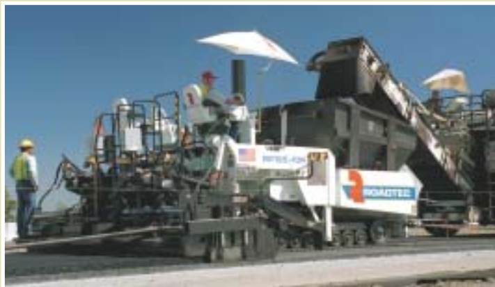
RP 185-10R rubber-track asphalt paver allows for maximum tractive effort.
