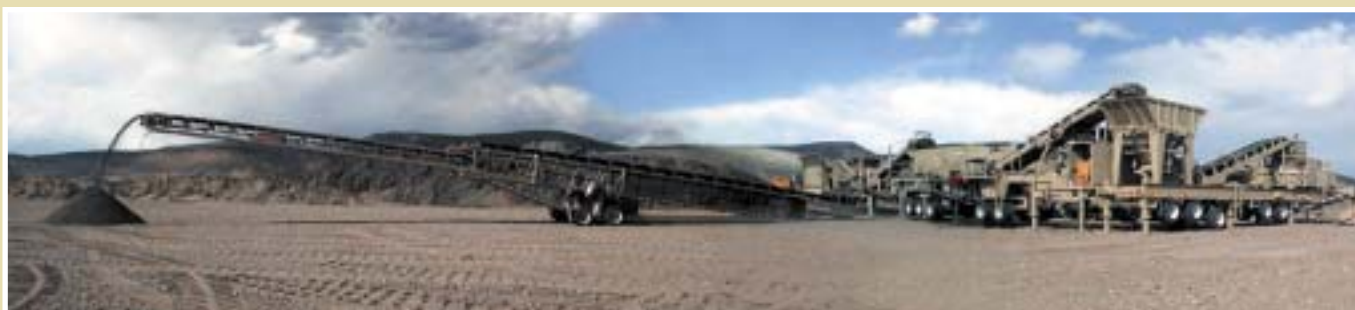
The Fast Pack® crushing spread in Colorado. This innovative plant sets up in under 5 hours and will produce 500 TPH of 6 spec products.
