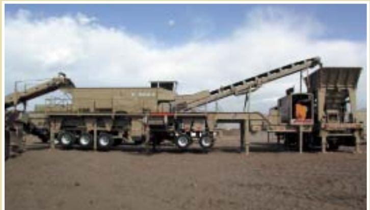
The Fast Pack® system uses on-board combination discharge/transfer conveyors that are hydraulically operated, requiring no support or extra loads.
