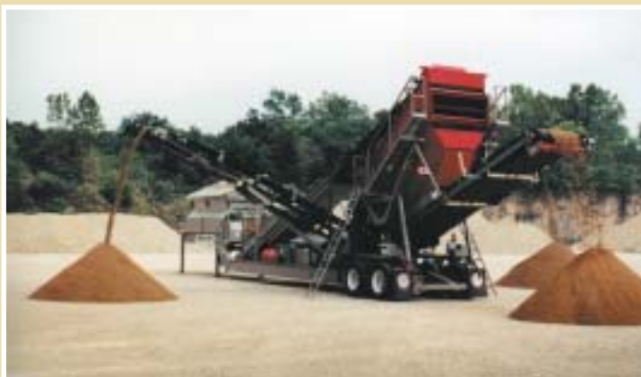
Fold N' Go® mobile screening plant.
