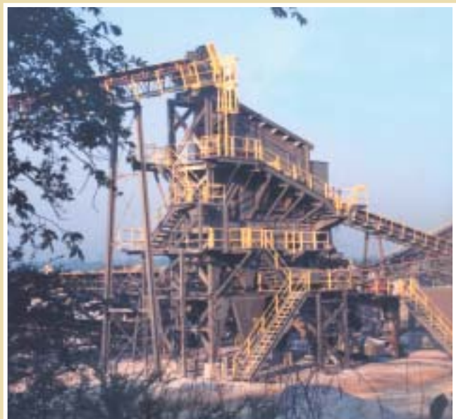
Dual-shaft 6' x 20' triple deck screen, on a modular tower with roll-away chutes, feeding a 52SBS cone crusher.
