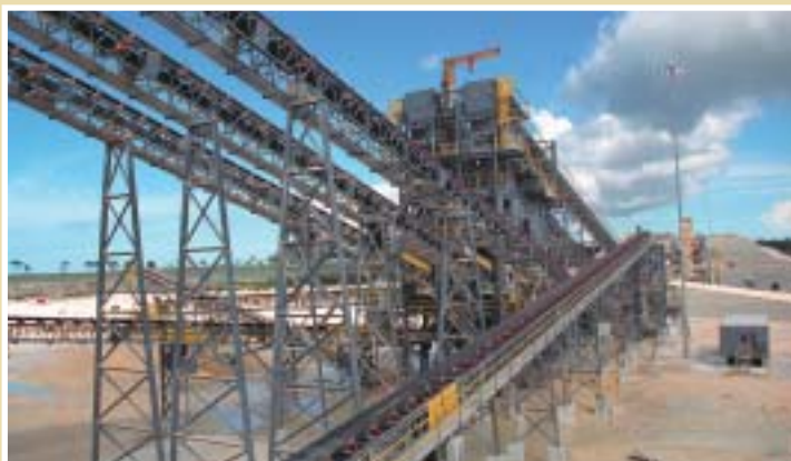
Modular twin dry screening towers in the Bahamas.
