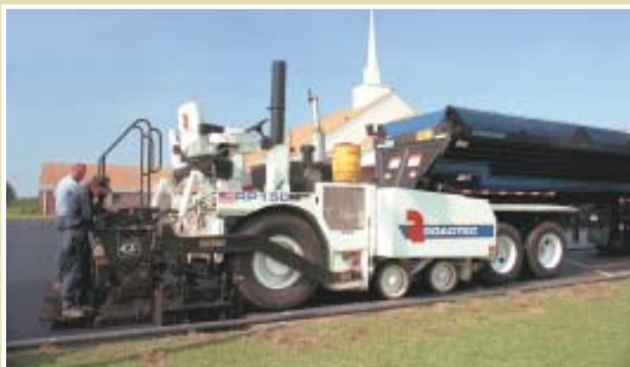
RP 150 asphalt paver features an 8 ft. paving width and shorter wheelbase.
