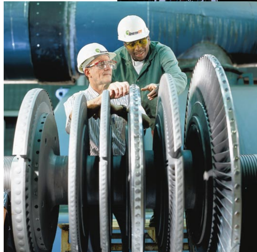
Engineer Richard Speraneo (left) and Craftsman Mark Newman are members of Coffeen Plant teams charged with overhauling a turbine and other equipment as part of an extensive outage at the AmerenCIPS plant. They are pictured here with the rotor of a recently refurbished drive turbine.
