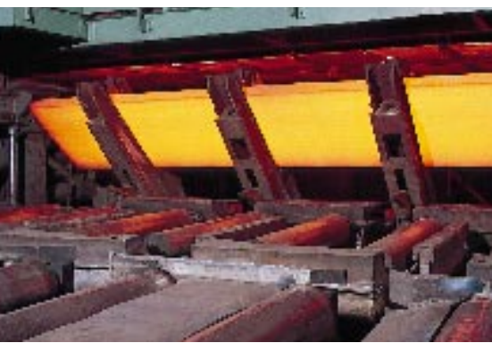
The induction furnaces at Allegheny Ludlum's Houston, PA plant are uniquely capable of reheating stainless steel, nickel alloys, titanium and zirconium slabs prior to hot rolling on the Steckel mill.
