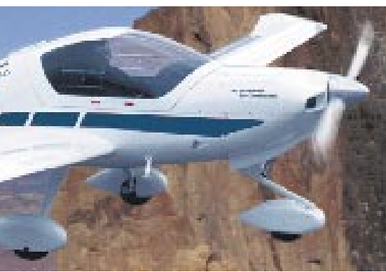
The Diamond Katana C1 Training Aircraft built by Diamond Aircraft Industries Inc. is one of four new advanced composite aircraft that were certified for production in 1998. Each new aircraft was certified with a Teledyne Continental Motors engine.
