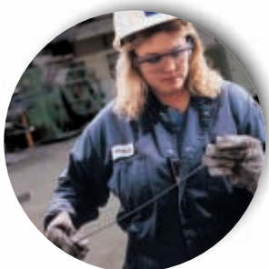
Wendy Whitt, wire draw operator, Wah Chang, performing the cold drawing processes of nickel-titanium (Nitinol), a shape memory alloy. This product is used to make a variety of medical grade products as well as cell phone antennas and eyeglass frames.
