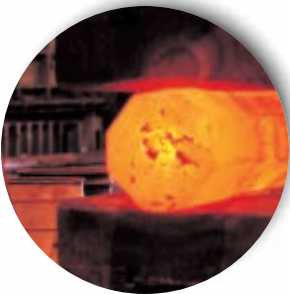
Hot titanium intermediate billet ready for press forging.
