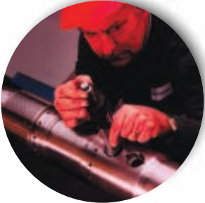
Staballoy AG17® non-magnetic oil tool being dimensionally inspected with a micrometer by Warrick Plummer, Allvac Ltd, U.K.
