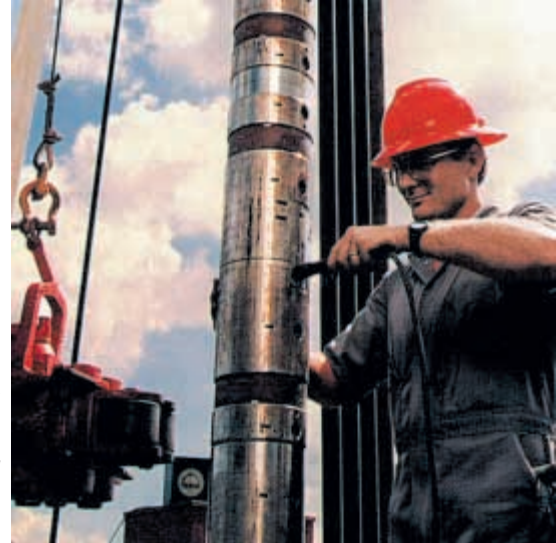
A Datalloy™ II MWD (measurement while drilling) collar, produced by Allvac Ltd, being assembled on a drilling rig.
