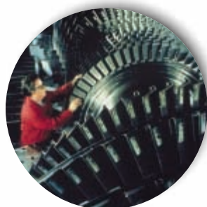
This land-based gas turbine being built by General Electric Power Systems uses Allegheny Technologies' nickel-based superalloys for turbine disk applications.
