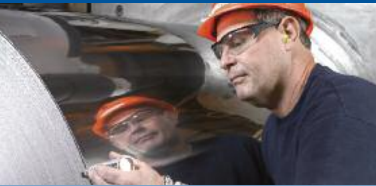
Left: Bruce Gula of ATI's Louisville, OH facility verifies the finish and gauge on a coil of specialty sheet on the plant's powerful Temper Mill, which imparts special finishes and strength levels. Our Louisville finishing operation produces a unique mix of titanium, nickel alloy, super stainless, and stainless sheet.
