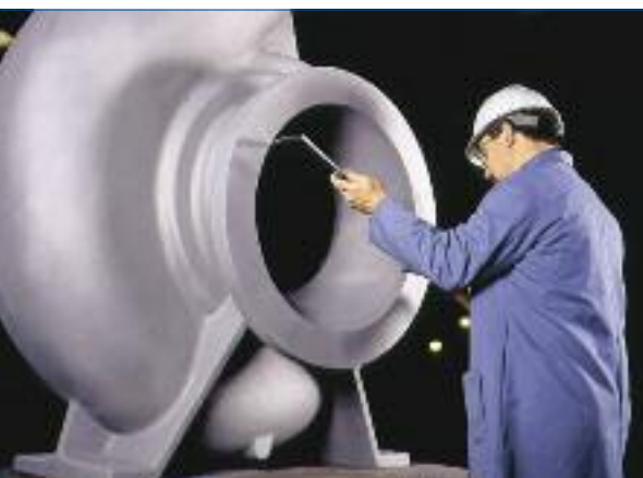
Above: Titanium for plate frame heat exchangers Below: Titanium and zirconium castings for pumps
