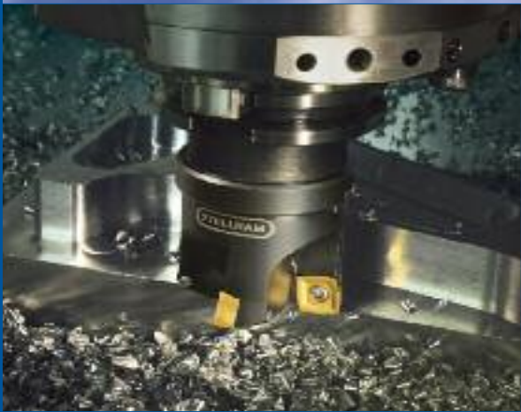
Above: High feed cutters for machining aerospace metals Below: Premium alloys for jet engine components
