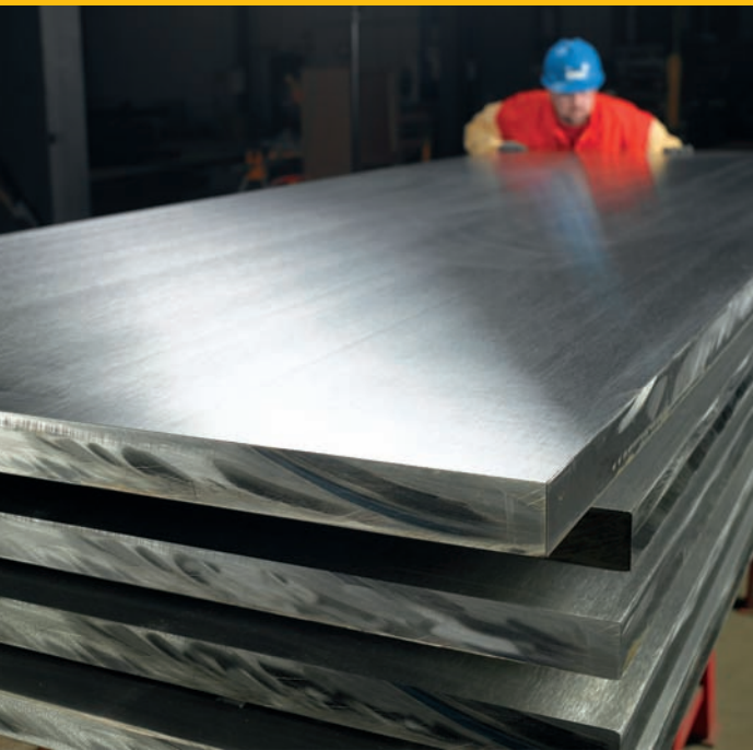
ATI 425® Alloy titanium plate undergoes final inspection after grinding by ATI Precision Finishing to assure proper surface and flatness before shipping to Aerospace and Defense customers.
