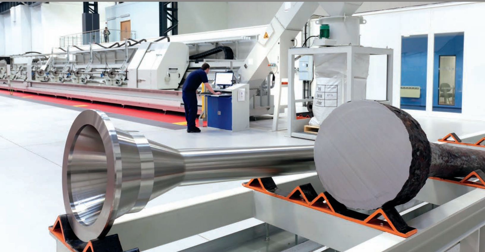
With a machined jet engine shaft in the left foreground and a near-net-shape forging to its right, Patrick Whitaker, an ATI precision machinist, monitors the collection of turnings from a CNC Deep Hole Borer at our Precision Machining Facility in Sheffield, UK. The turnings are captured and returned to ATI's Latrobe, PA, operations for recycling.
