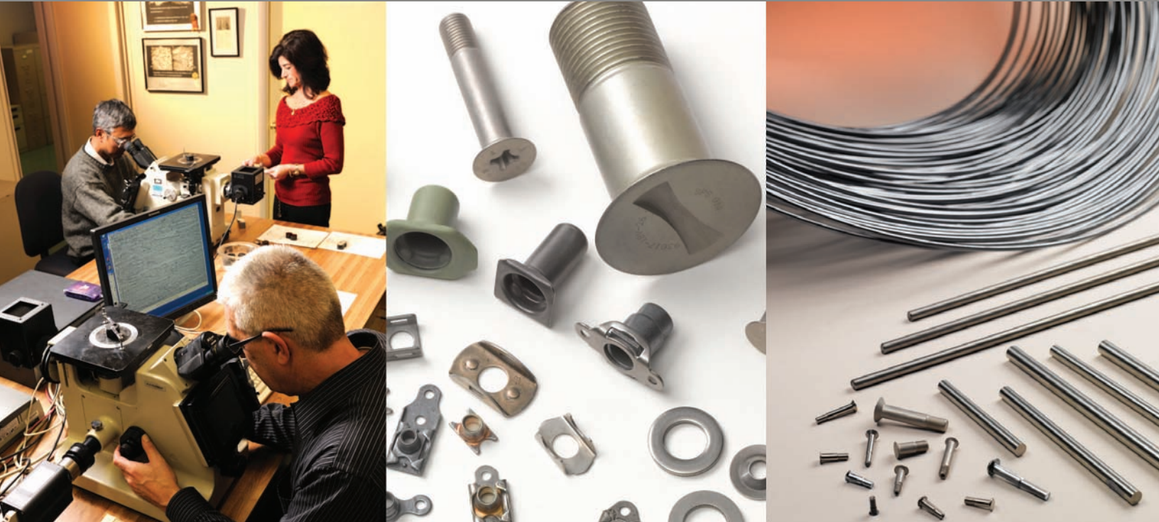
Left to right: ATI Metallurgist Bill Pelican (foreground) adjusts the microscopic image of the grain structure of a cross-section of ATI 425 ® Alloy cold-rolled titanium sheet for evaluation by Cheryl Botti, the marketing leader for ATI 425 Alloy sheet products, with Tom Parayil, leader of ATI's physical metallurgy group; ATI provides a broad range of material solutions to aerospace fastener manufacturers; ATI's titanium bar, rod, and coil are used to produce aerospace fasteners.
