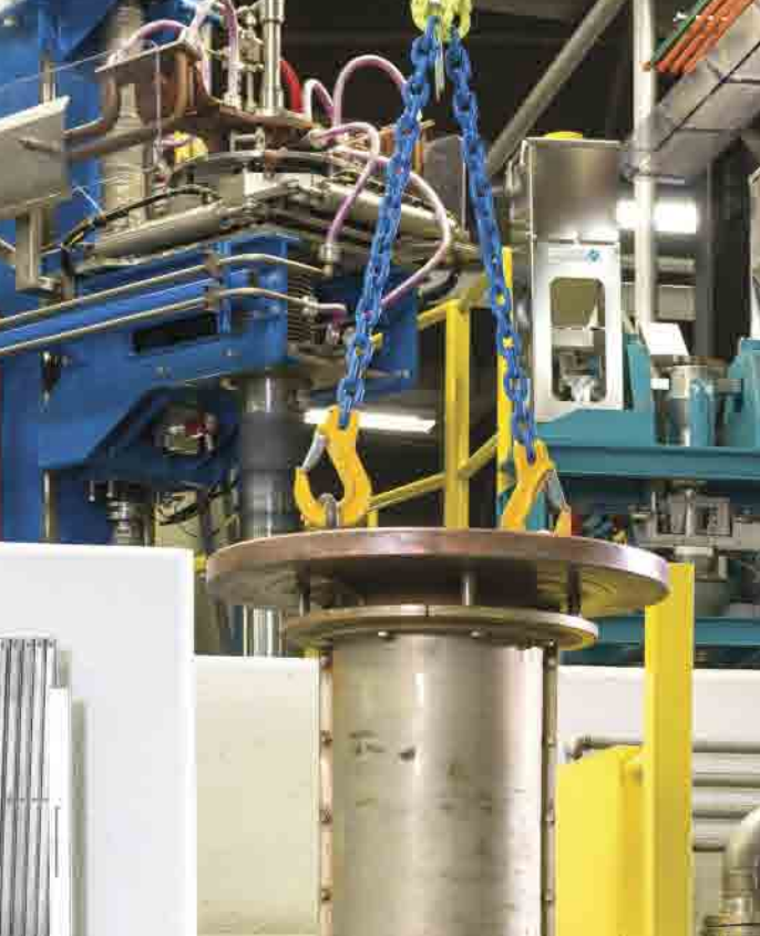
ATI Specialty Materials Pilot Plant Melter Corey Hines examines a 10-inch diameter ingot of a new titanium alloy upon its exit from a crucible belonging to the company's ESR / VAR R&D furnace. The larger ingots produced by the furnace enhance both the productivity and validity of the experiments on titanium and nickel-based alloys and production processes.
