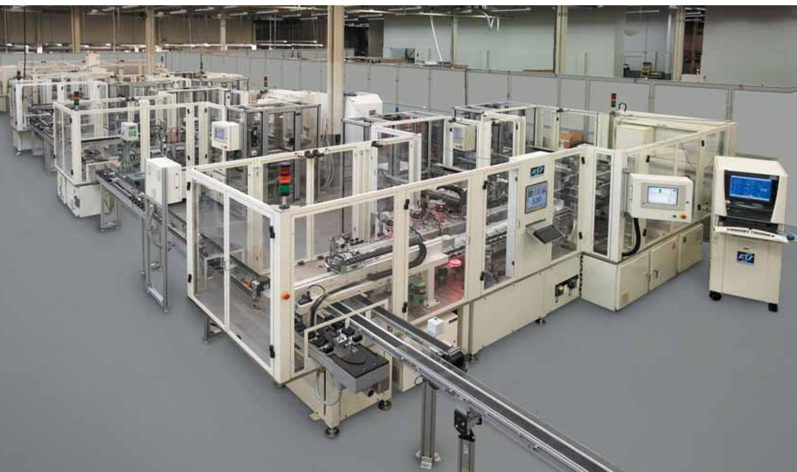
ATS designed, built and installed this innovative automation system in fiscal 2005 to produce and test a sophisticated medical diagnostic device. The system is a showcase for ATS standard technology platforms and includes ATS SuperTrak™, ATS Trayhandler™, Superbot™ robotics, ATS MACS™ machine control software system, Production stATS™ optimization program, and an ATS flexible feeding system.
