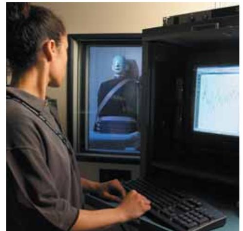
A PCG technician uses specialized acoustic testing equipment to check for mechanical sound levels within a highly engineered automotive seat component. PCG serves several of the world's largest automotive customers.
