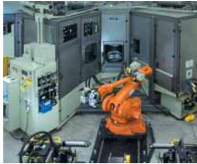
ATS Rotoper™ Flexible Rotary Transfer System is a sophisticated heavy-duty precision machining system that delivers maximum throughput for a wide range of materials including aluminum, steel and cast iron. Here, a material handling system is shown loading a cylinder-head casting into the machining centre.
