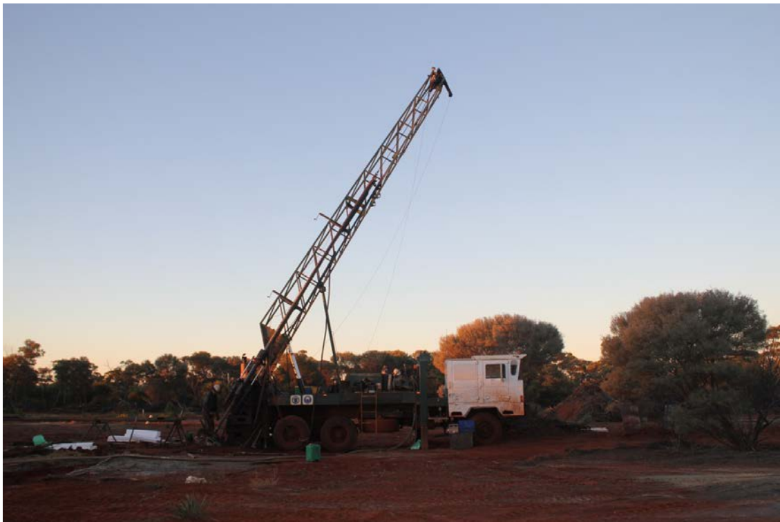
Diamond drill rig in operation at Halleys East – June 2012
