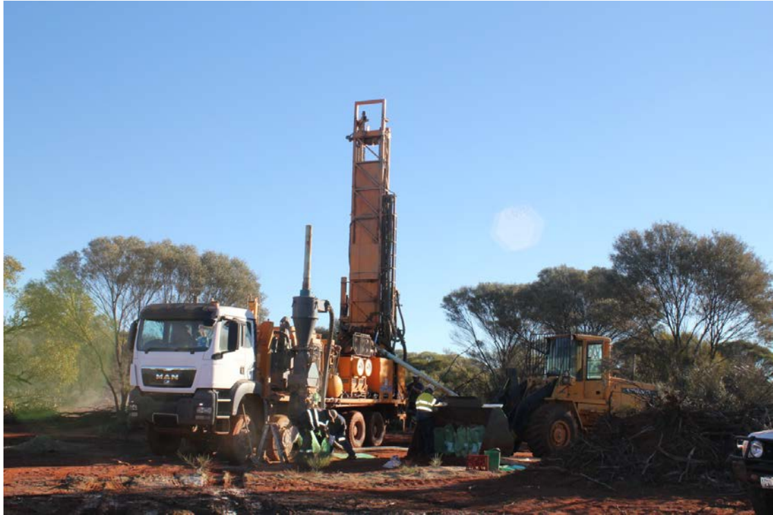
Percussion drill rig in operation at Halleys East – June 2012
