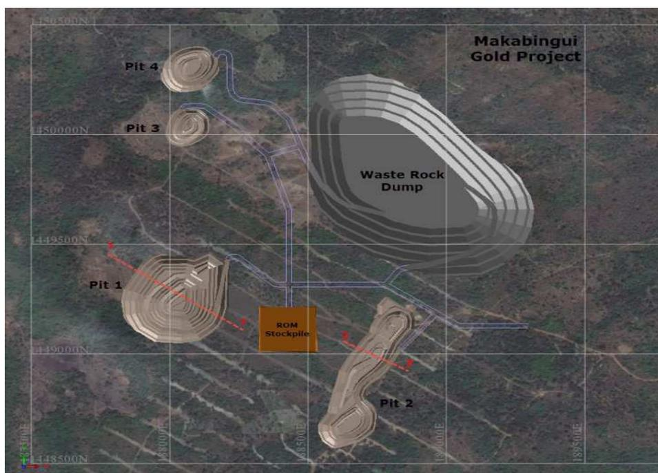
**Figure 2 - Mine Plan View Showing Pits and Waste Dump**
