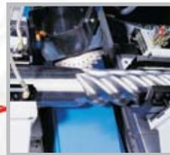
The steel is then machined into the rotor shape required for down-hole drilling
