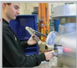
The HIPed and heat treated NNS shape valve body is laser scanned to compare the dimensions of the actual component with the NNS product drawing
