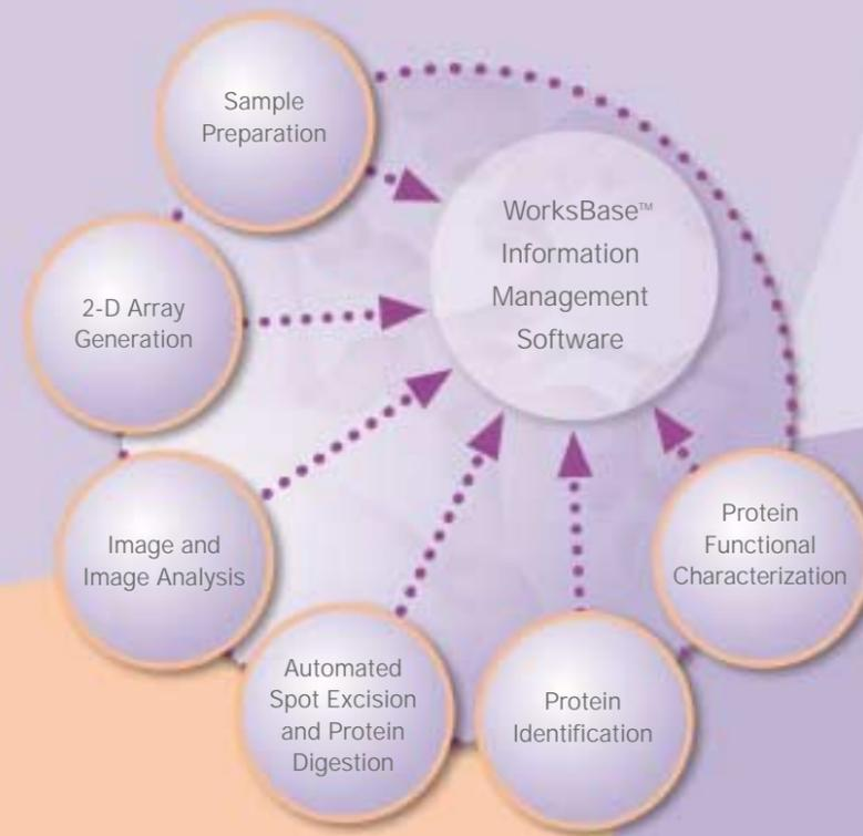
Bio-Rad's ProteomeWorks™ System is a fully integrated set of tools and technologies used for protein function discovery, incorporating sample preparation, 2-D electrophoresis, staining, imaging and image analysis, spot excision, automated protein digestion, mass spectrometry and bioinformatics to create a seamless high-throughput proteomics platform.
