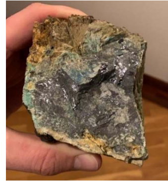
FIGURE 7: Mestersvig Project, rock chip sample 4958 showing massive galena hosted in a quartz vein.
