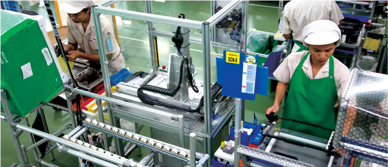
“Man-machine cell” production systems integrate processes where robots excel with processes that can only be performed by people to sharply enhance the productivity of cell production systems. (Canon Hi-Tech Thailand Ltd.)
