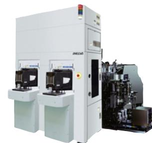
**The FC7100** system enables ultrathin film composition in an ultrahigh vacuum and so contributes to the rapid growth of mobile handsets as a technology that is indispensable to making devices smaller and more energy efficient.
