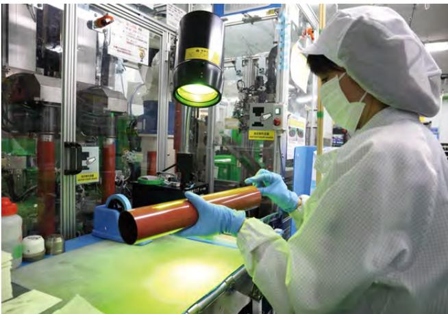
**In-house production:** Canon-developed fixing belts for copiers are produced in Japan. (Toride Plant)
