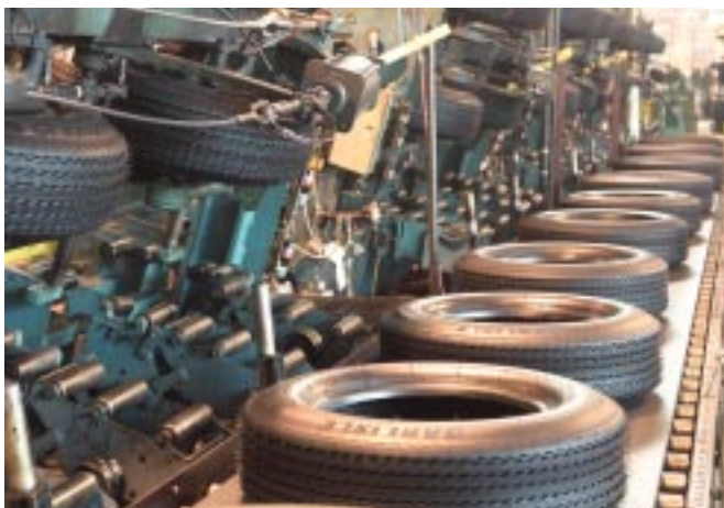
Finished tires are conveyed behind the curing presses at Carlisle Tire & Wheel
