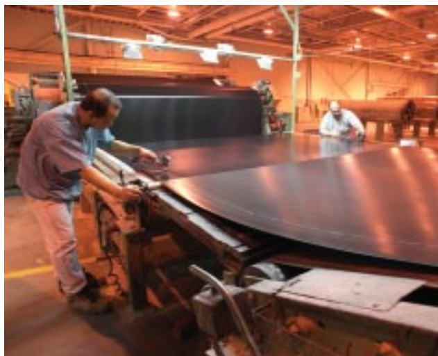
Dimensional checks are completed on a 60 millimeter thick membrane at Carlisle SynTec
