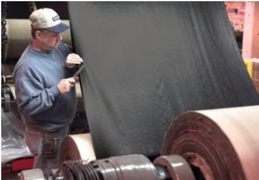
Nylon cord that will become tire plies is coated with rubber at Carlisle Tire & Wheel
