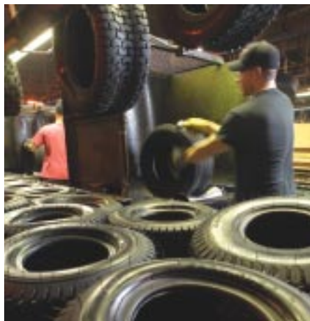
Excess rubber is trimmed from the tires after molding at Carlisle Tire & Wheel
