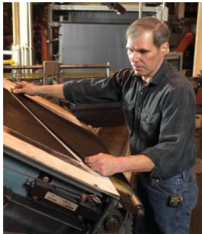
Rubber coated nylon plies are cut to a precise angle and width at Carlisle Tire & Wheel
