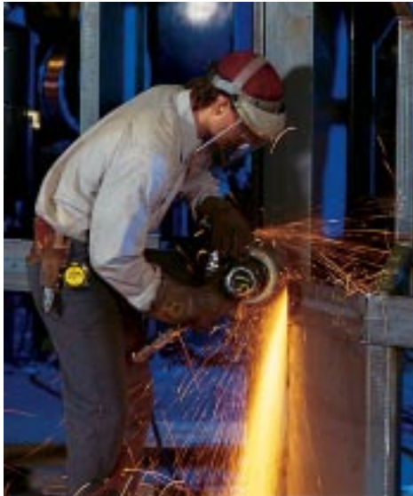
Grinding joints on a Trail King truck body
