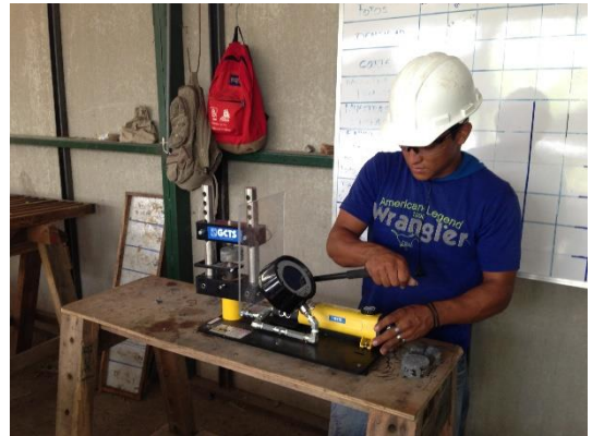
Figure 11. Point load testing geotechnical drill core samples.
