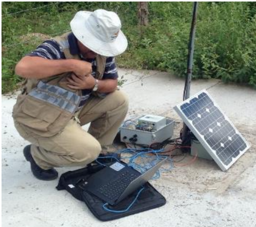
Figure 5. Ongoing collection of base-line meteorological data at La India as part of the EIA studies.
