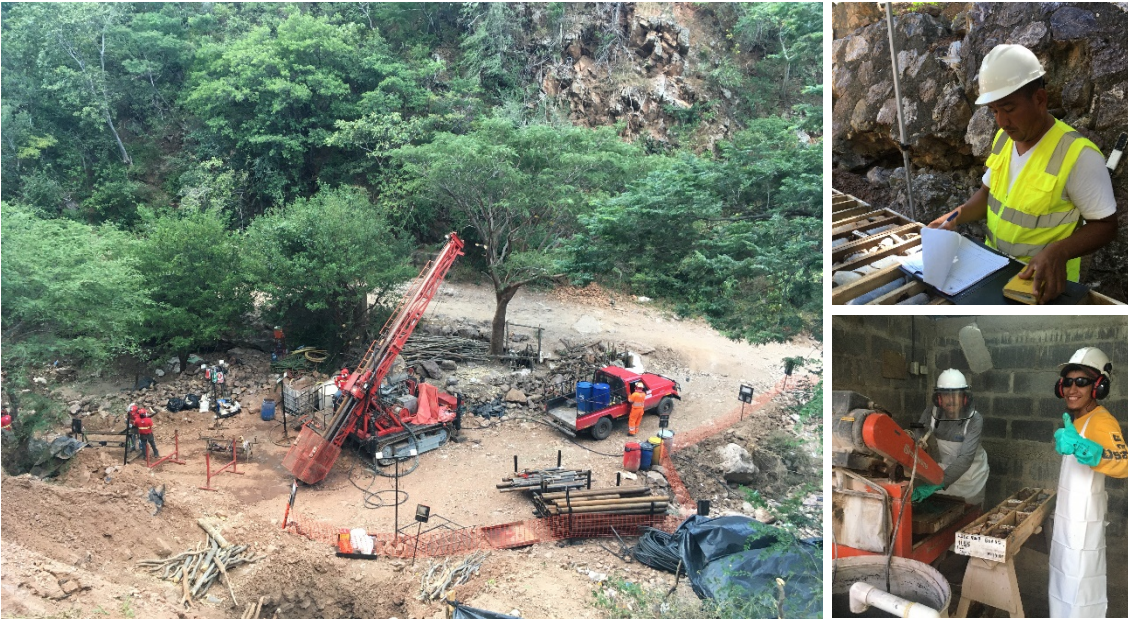
Drilling the first drill hole of the La India starter pit infill programme (left); the geologist logging the core (top right); and geological assistants cutting and sampling core (bottom right). Drill hole LIDC404 was collared in the main historic mine zone and tested the thickness of the un-exploited footwall mineralisation within the planned starter pit in the high-grade Northern Zone of the La India Vein.
