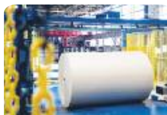
CCM reels are shipped from the paper mill to a box plant for conversion into corrugated board.
