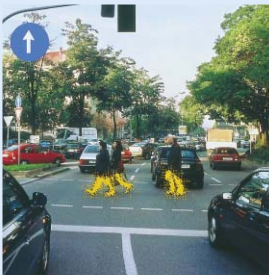
Pedestrians are recognized from their typical leg movements. The system uses picture sequences for identification.
