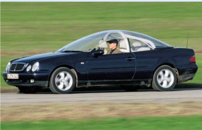
The CLK convertible with a glass bubble roof is used to investigate vision requirements when driving. The test drivers' viewing behavior can be analyzed with a variety of simulated A columns.
