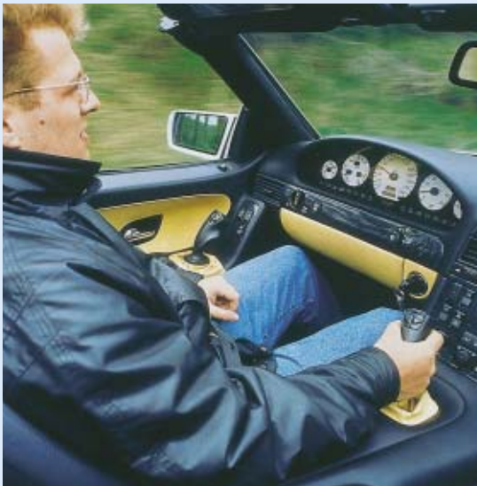
Proven in the test car: In critical situations a driver can react faster with sidesticks than with accelerator and brake pedal.
