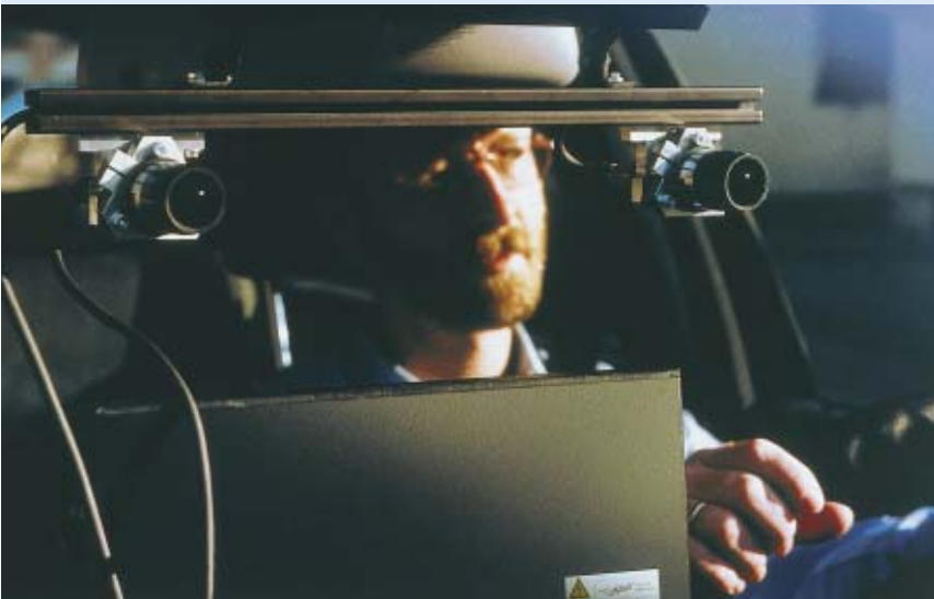
The stereo-vision camera is the sensor for the City Assistant. The picture of the surroundings must be passed on in high definition to image processing for instant evaluation.
