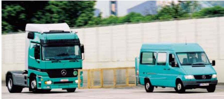
The automatic emergency braking system, Protector, first gives the driver an acoustic and visual warning of an imminent front-end collision. If he does not react, the system decelerates the truck with maximum braking force.
