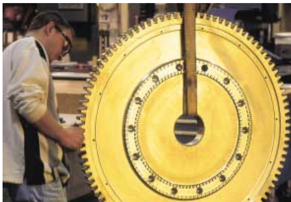
A turbine disk, manufactured by MTU Aero Engine Components
