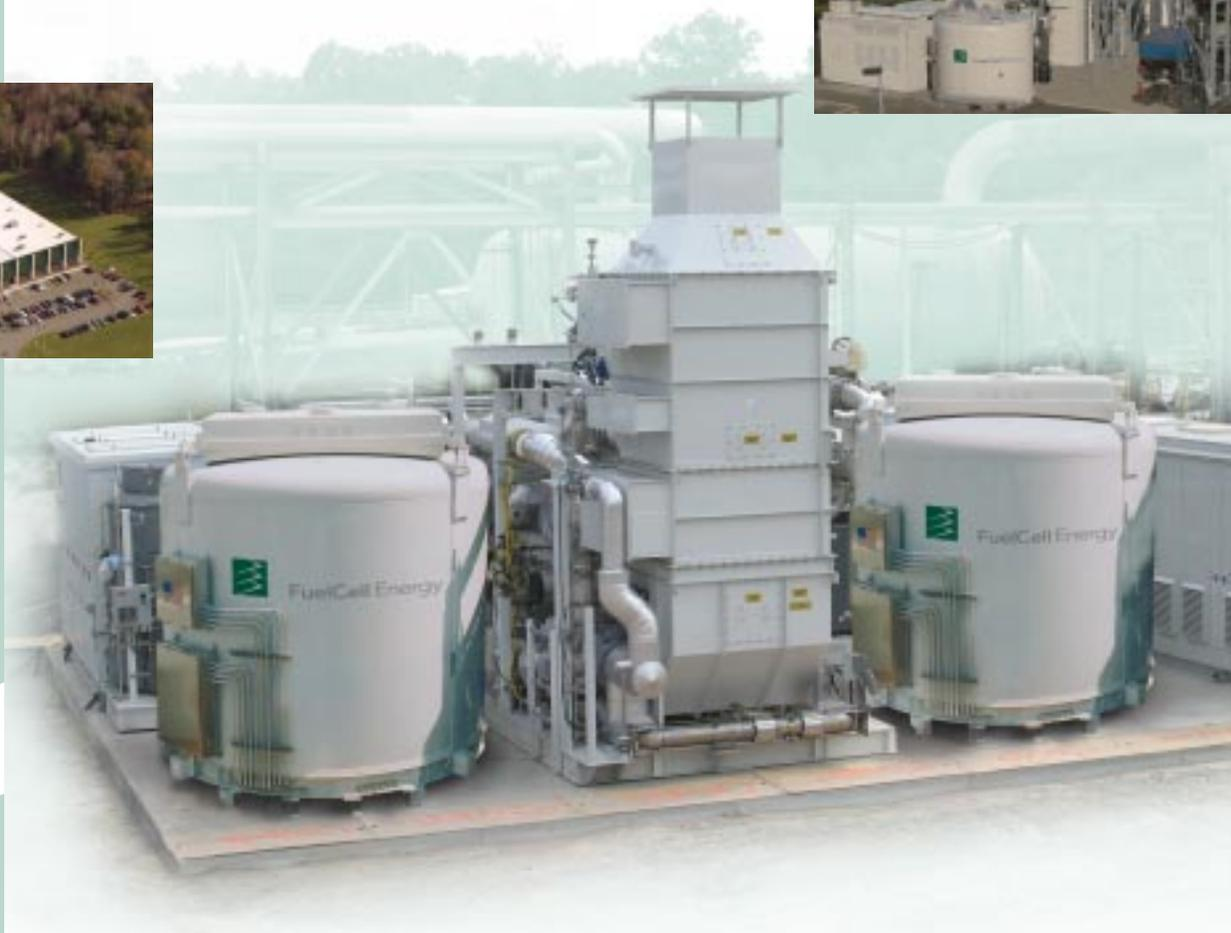
FuelCell Energy's first 2 MW DFC3000 power plant operates on both natural gas and synthesis gas from a coal gasification plant in Wabash, IN.
