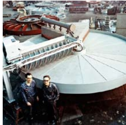
FLSmidth Dorr-Oliver Eimco sedimentation filter in production.
