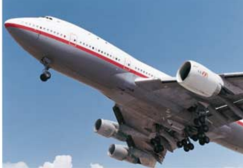
1999 flight testing of a growth GE90 engine, installed on GE's unique 747 flying testbed, marked a significant milestone in the GE90-115B development program.
