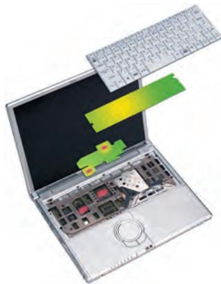
eGraf® materials eliminated the need for fan, heat pipes and heat sinks.
