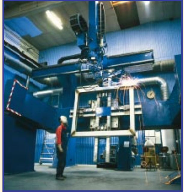
Welding the reinforcement channels in the new welding robot.
