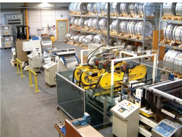
Holders Technology GmbH is a leading supplier of the aluminium sheets used in PCB manufacturing. Sheets are cut to size from giant rolls, shown here: visit [www.holderstechnology.com](http://www.holderstechnology.com)
