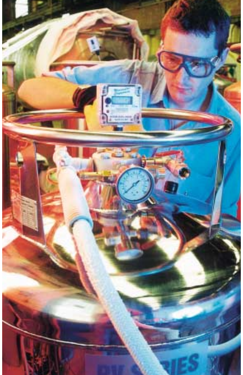
In an emergency, Elfab bursting discs would safely release excessive pressure from these Wessington Cryogenics Ltd gas storage vessels.
