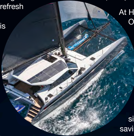
Hexcel composites provide stiffness without adding weight to the Gunboat 68. Photo courtesy of Gunboat.
