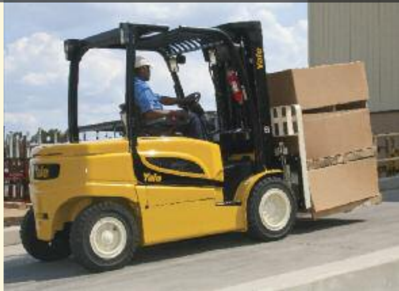
One of Yale's electric counterbalanced lift trucks, the Yale® ERP100-VM four-wheel pneumatic tire lift truck series, with a lifting capacity of up to 10,000 pounds, was launched in mid-2013.
