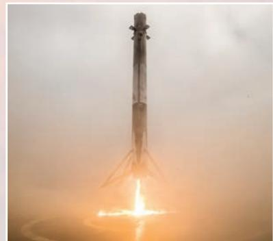
SpaceX's launch program was developed for rocket reusability. The images directly above and below show the landing of the first-stage rocket following the successful launch of Iridium NEXT satellites on June 25. This same first-stage was used on December 22 to launch another batch of Iridium NEXT satellites to space.
