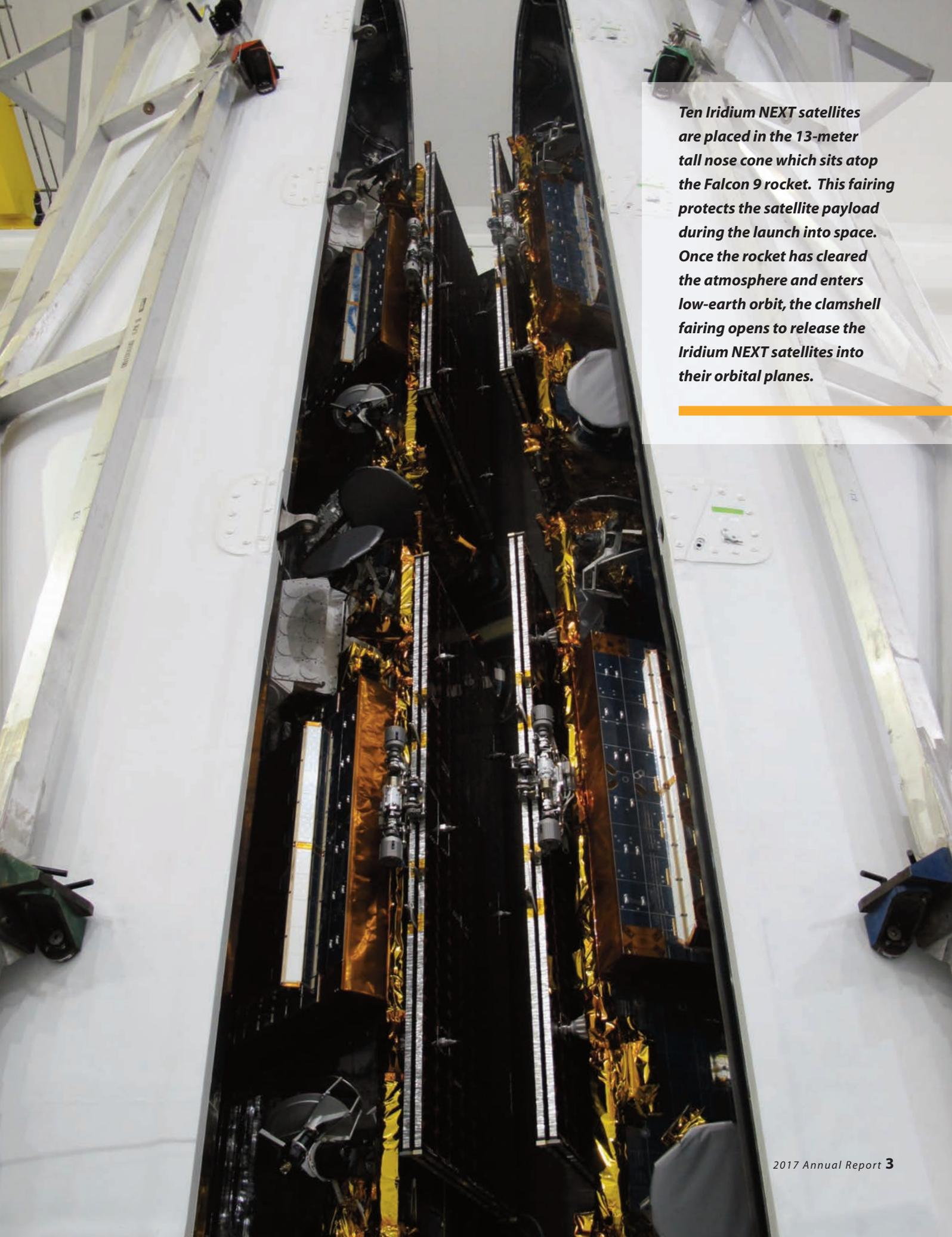
*Ten Iridium NEXT satellites are placed in the 13-meter tall nose cone which sits atop the Falcon 9 rocket. This fairing protects the satellite payload during the launch into space. Once the rocket has cleared the atmosphere and enters low-earth orbit, the clamshell fairing opens to release the Iridium NEXT satellites into their orbital planes.*
