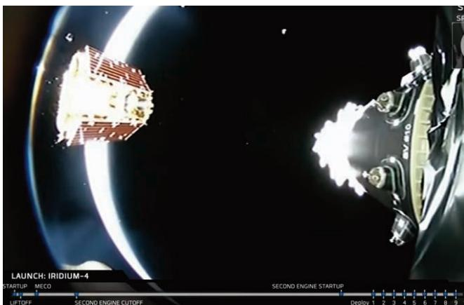
*As satellites fall away from the dispenser ring, they travel at a speed of approximately 17,000 miles per hour and will begin several weeks of testing in orbit prior to insertion in the Iridium network, where they will carry live customer traffic.*
