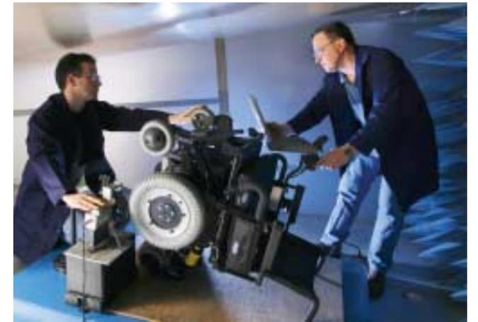
**Testing.** Invacare associates test the electronics on a new power wheelchair. The anechoic testing chamber is lined with radio-frequency absorbing material to reduce reflections from internal surfaces.
