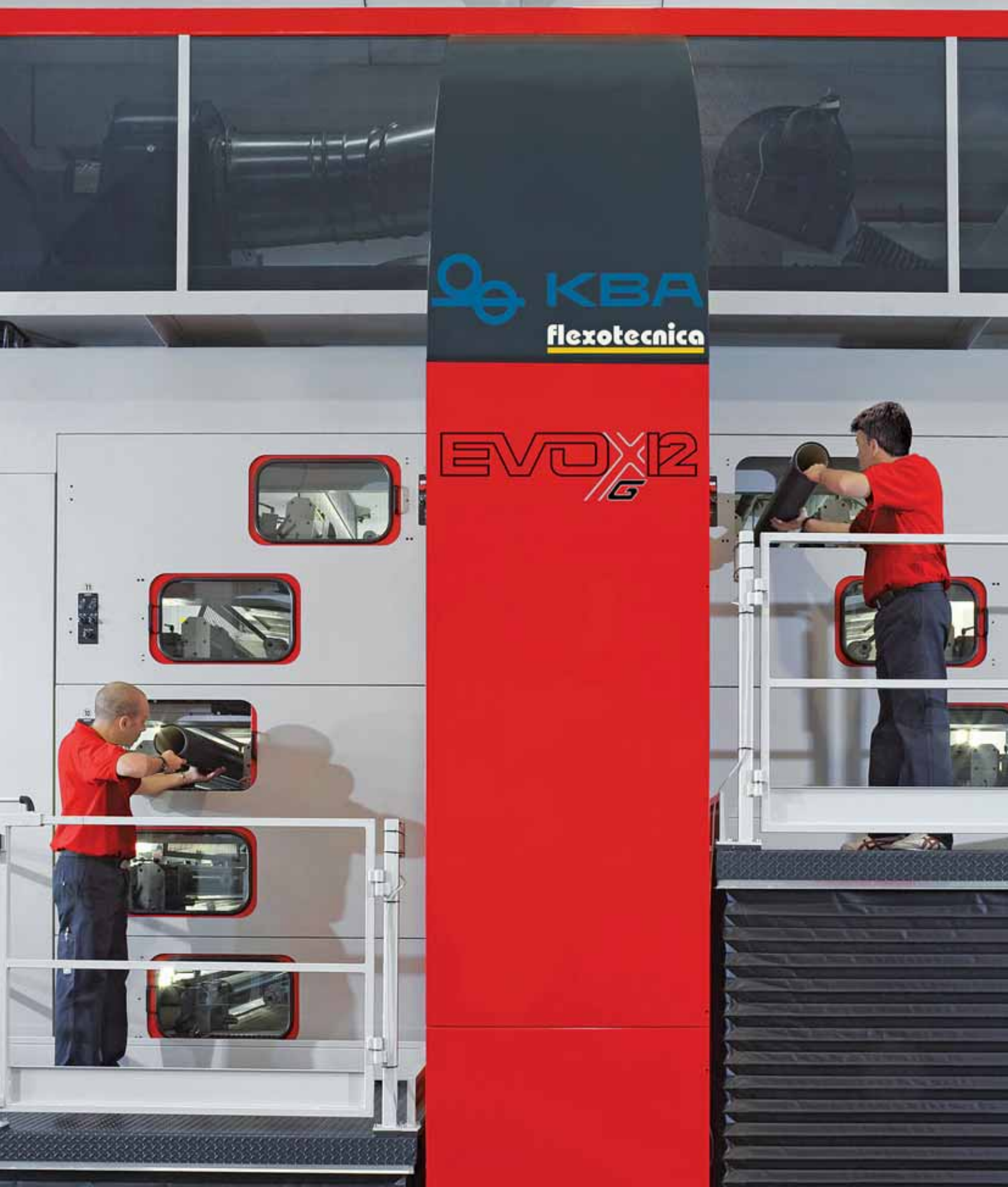
The EVO XG 12 from KBA-Flexotecnica featuring 12 print decks, printing widths of up to 2m and speeds of up to 600m/min is our Italian subsidiary's leading product for the flexible packaging market
