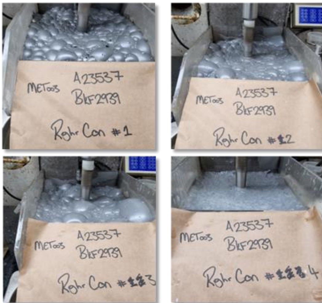
Mt Felstead Prospect rougher flotation concentration stages one to four
