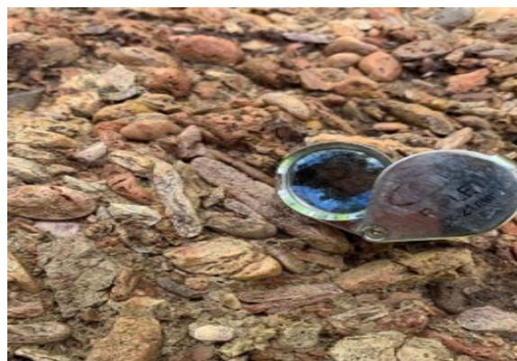
**Figure 2: Bouba Plateau Conglomerate Bauxite**
