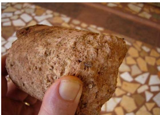
**Figure 1: Typical Insitu Bauxite**
