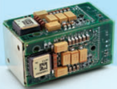
Interior of VectorSeis sensor
