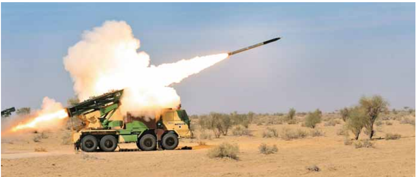
Multi-barrel rocket-launch system for India's defence forces, designed and developed by L&T - largely through in-house R&D.
