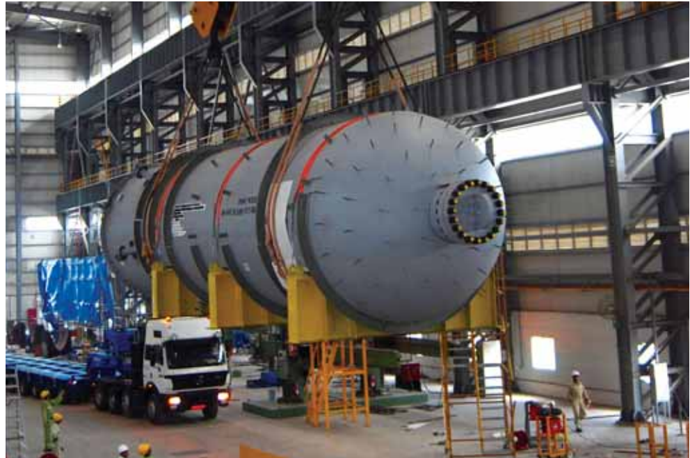
Cr-Mo HDS reactor manufactured at L&T's works complex in Sohar, Oman. The complex includes a captive jetty having direct access to the Gulf of Oman.
