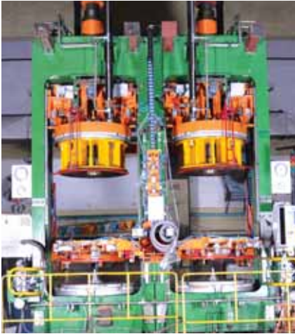
Hydraulic tyre-curing press, manufactured by LTM BU. It is used by tyre suppliers to manufacture passenger car radial tyres.
