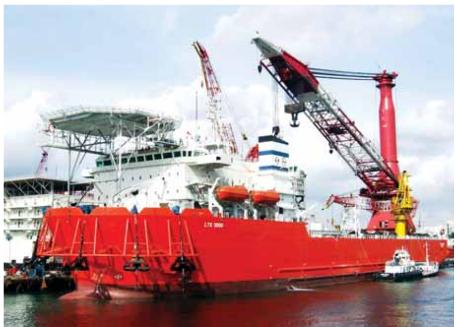
290-man 3000 ST heavy-lift-cum-pipelay vessel (LTS 3000) adds installation capabilities to L&T's EPC offerings to the upstream hydrocarbon sector.
